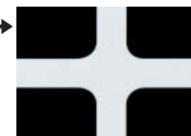
The target in the viewfinder allows easy manual focusing.
